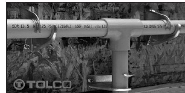
Tolco Stand-Off Hanger/Restrainer can function as a hanger or as a restrainer for installations where a standard offset is required. The Stand-Off Hanger can perform as both a hanger and restrainer on horizontal piping, and as a stabilizer for vertical sprinkler head drops. The manufacturer furnishes listed fasteners for use into wood.
