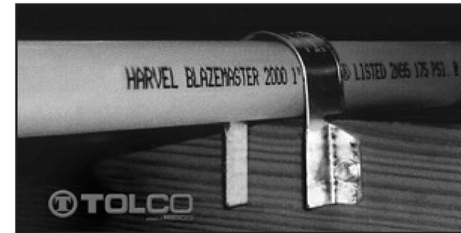
Tolco Hanger/Restrainer can function as a hanger or as a restrainer and can be mounted from the top or bottom of a beam. The fastener mounting edges are designed to allow the screws to be installed horizontally. This is a benefit when overhead clearance is limited.
